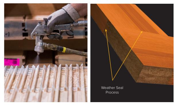
Finally, all Simpson Performance Doors come with a solid bottom rail. Solid lumber is very durable especially in this vulnerable area of the door. By incorporating all three of these into a door, the entire bottom of the door is protected against moisture penetration.
